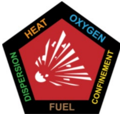
Figure 1: The dust deflagration pentagon. Note the three legs of the combustion triangle.
