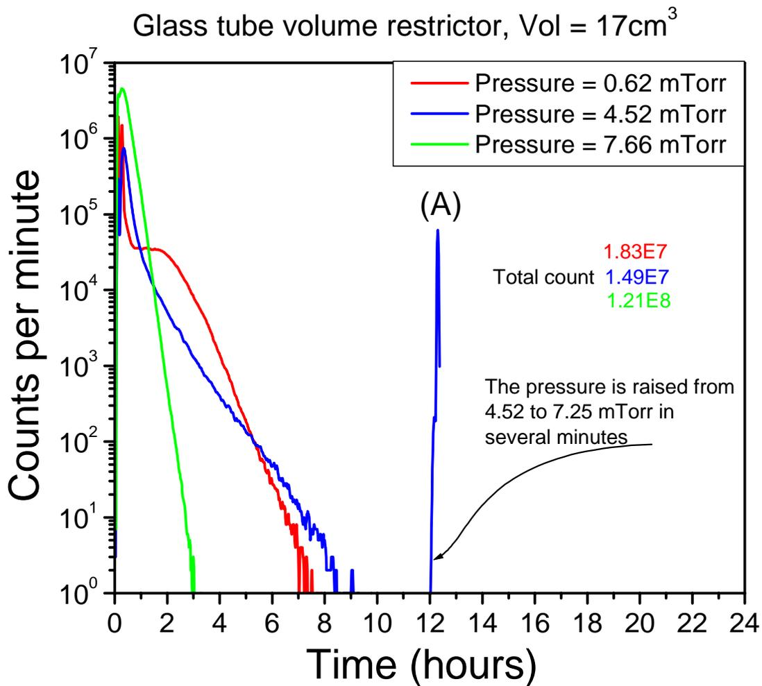
Here we show the effect of pressure on how long the crystal will produce electron after it was heated to 150 °C and left to cool. The peak at the point marked (A) is the result of increased electron production when the pressure was raised from 4.52 mTorr to 7.25 mTorr.
