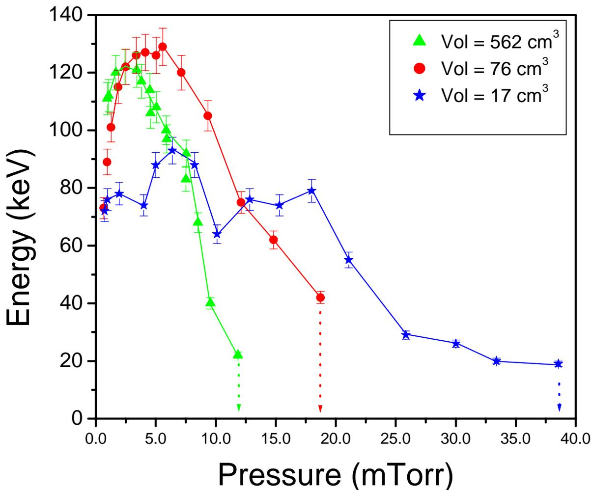
Here we show the effect of reducing the effective volume around the crystal without changing the size of the vacuum chamber. We attempted to assure pressure equilibrium by waiting for not less than 30 minutes between pressures changes and 24 hours between changes in volume restrictors.
