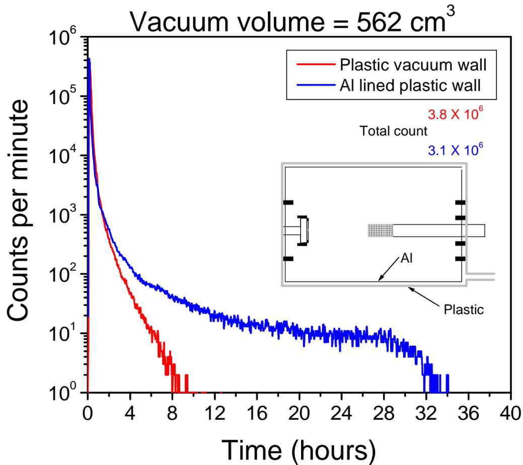
Here we show the effect of lining the **plastic** vacuum chamber wall with **Al** foil. The Al foil is grounded. The +Z base of the crystal was heated to  $\sim 150 \text{ }^\circ\text{C}$  and left to cool to room temperature. Data was collected until the count rate fell to about 1 count per minute.
