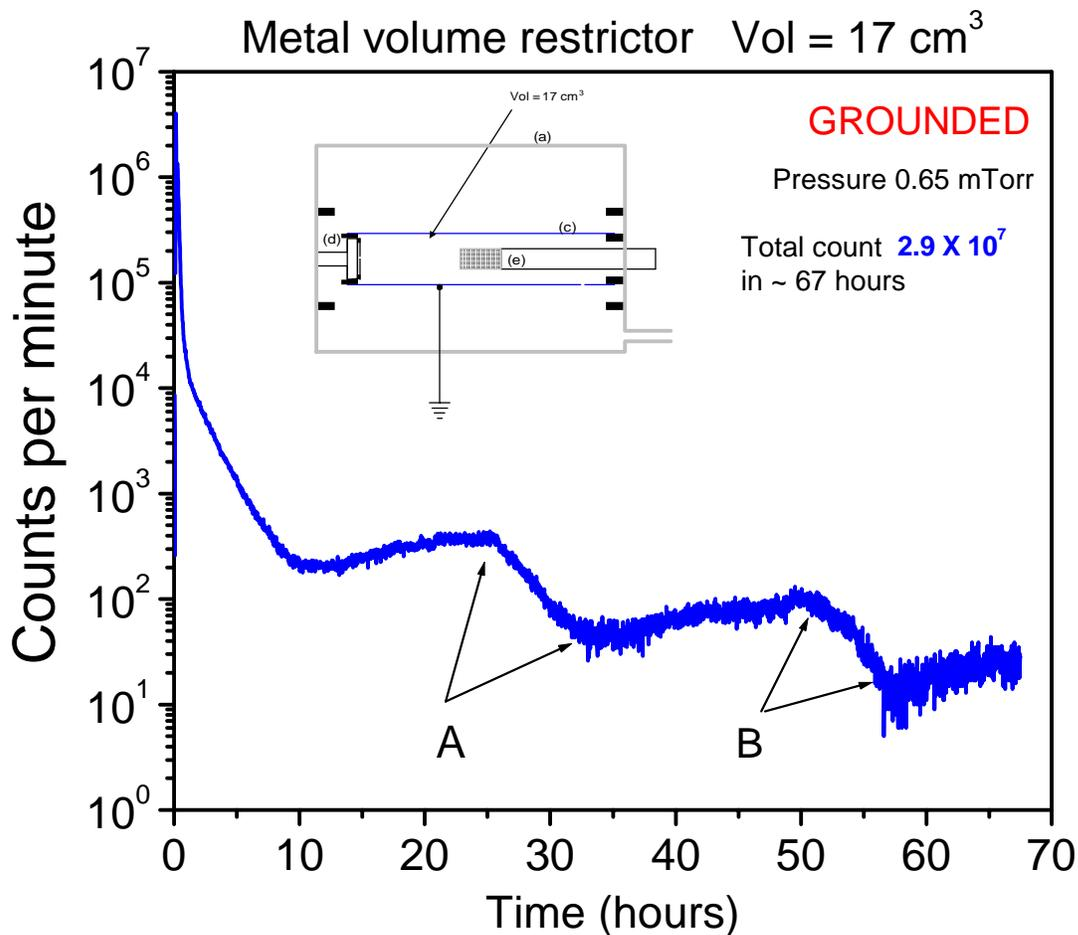
Here we show the effect of a **grounded** metal volume restrictor. The +Z base of the crystal was heated to  $\sim 150^\circ\text{C}$  and left to cool to room temperature. Data was collected for more than 67 hours. The change in count rate at **A** and **B** is believed to be caused by a large change in room temperature between night and day.
