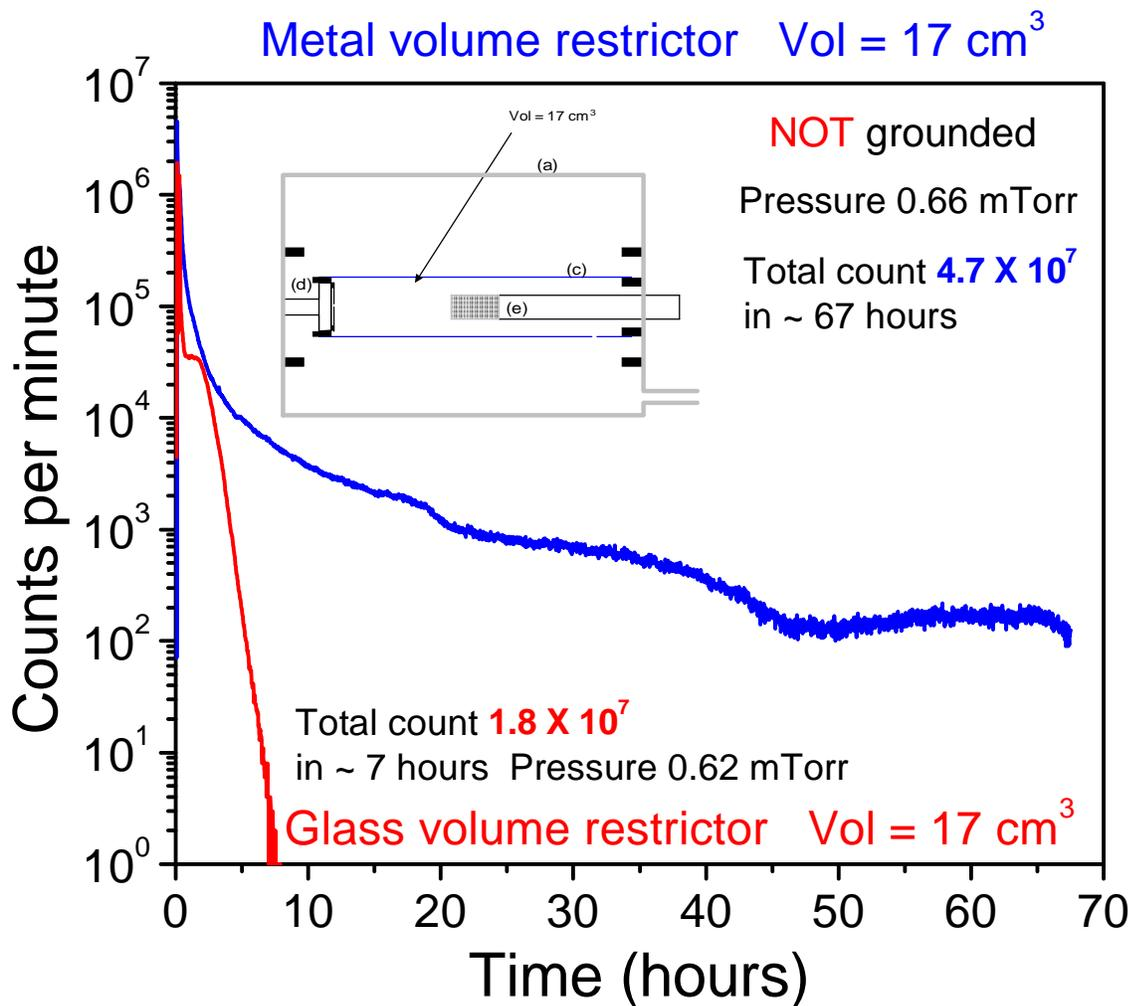
Here we show the effect of an **ungrounded** metal volume restrictor. The +Z base of the crystal was heated to  $\sim 150$  °C and left to cool to room temperature. Data was collected for more than 67 hours. The **red** trace shows what happened when the metal tube is replaced with a glass tube.
