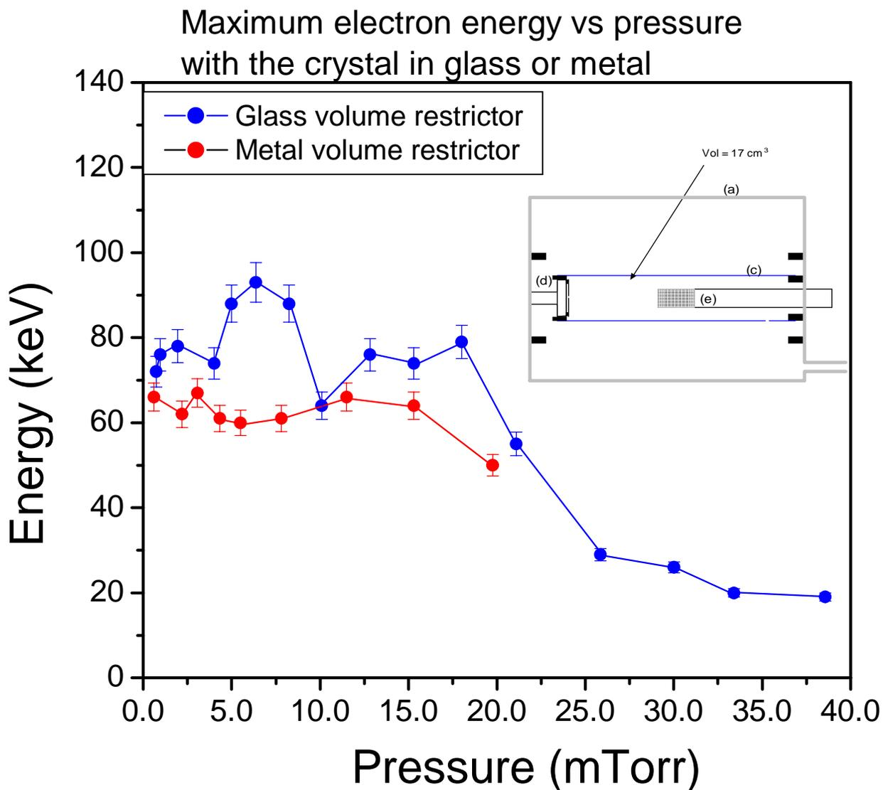
Here we show the effect of using glass vs. metal as a volume restrictor around the crystal. The maximum energy is less when metal is used and the maximum pressure at which the crystal will produce electrons is also less. There were several discharges during runs with the glass tube. A discharge reduces the maximum electron energy.
