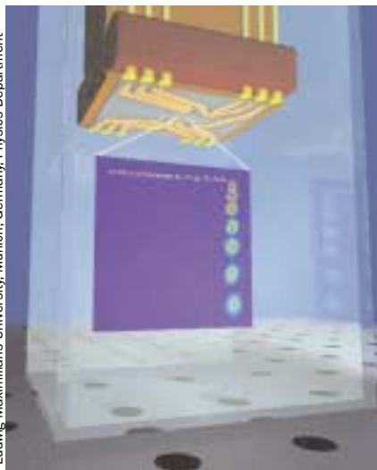
In this computer graphic of a microchip upside down in an ultrahigh-vacuum glass cell, the BEC is produced on the left, transported to the right, and released into free-fall, showing the characteristic spherical cloud of atoms (blue) with a dense elliptic center (red and yellow).
